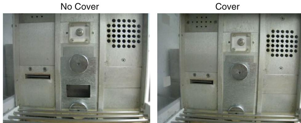
**Fig. 1** Pictures of the apparatus configurations in the No Cover (*left panel*) and Cover (*right panel*) conditions. In the Cover condition, a metal plate blocked access to the drinking receptacle
